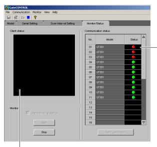
Indicator for the communication status with the connected device Green: Normal (comm. open)
