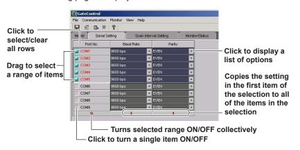
2. Turn ON the port numbers to be used, and set the baud rate, and parity.
