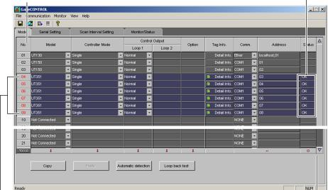
Drag to select a range for collective setting or the loop back test
